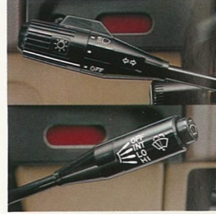
Light & wiper/washer controls on column. Intermittent wipers are part of set option on Wagon with tilt steering wheel.
