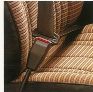
Optional ELR (Emergency Locking Retractor) seatbelts allow for more freedom of movement.
