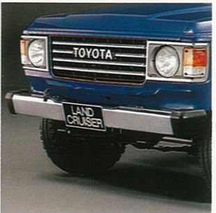
The corner rubbers and steel bumpers protect the body. There are two types of bumpers: optional chrome, and grey-painted steel.
