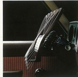
Optional tilt steering adjusts to 6 positions upward and down.
