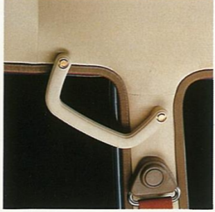
Optional rear ride-on grips help passengers get in and out of the back.
