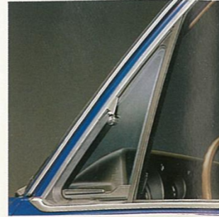
The flip-out front quarter windows (option) provide air circulation throughout the Station Wagon.
