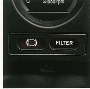
Filter lamp tells you when the water in the sedimenter reaches 200cc. Standard on Diesel models.
