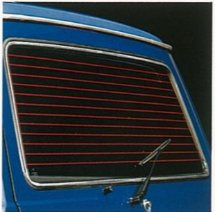
Rear window wiper and defogger (option on Wagon G and GX) always keep rear view clear.
